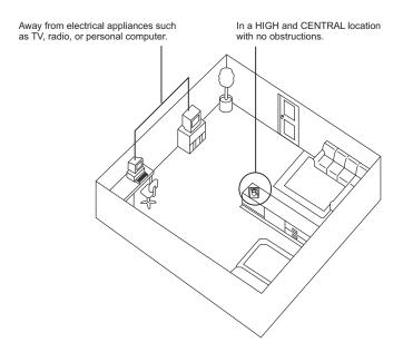
Do not place the base station on top of or near TV or VCR as this may interfere with the performance of these appliances.
